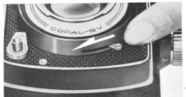
When using the self-timer, always see to it that the Flash Synchronizer Selector is switched to "X" position.
