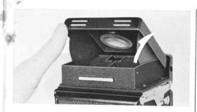
The exposure meter begins to function when the focusing hood is set upright by lifting it up gently with your fingertip.
